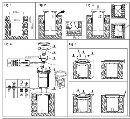
**Decking Fitting** - If fitting this product in decking subject to foot traffic then we would recommend that CFL or LED bulbs are used. If a halogen lamp is required then a 20W lamp should be fitted.
