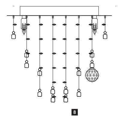
Voltage: 230V - 50/60Hz Lampholder: G9 Lamps: 5 x 33W Max
