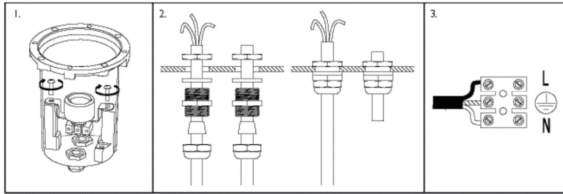
7. Undo the two screws holding the lampholder in place and lift out. You may also need to undo the earth screw on the body as well.
