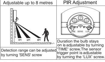
To access the adjustment screws flip down the black cover over the PIR sensor. Take great care when adjusting the sensor screws not to overtighten as they can be easily broken.
