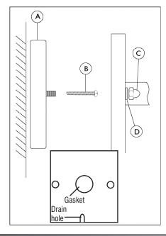
Thread the cable through the hole, ensuring the drain hole is at the base of the mounting box.
