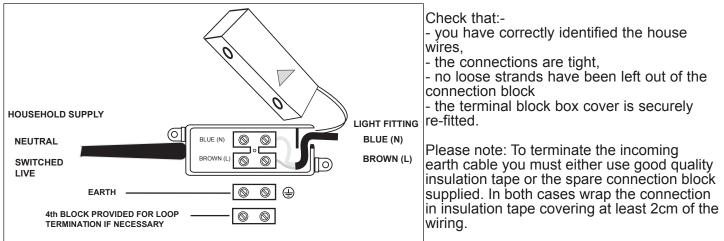
A fourth connection block is provided should you need it to make loop connection. You must then wrap the connection block in tape covering at least 2cm of the wiring on each side.
