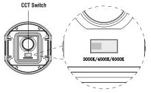
This product is colur changing and can be either warm white (3000K) or cool white (4000K) or daylight white (6000K). Choose your preferred colour before installing by using the CCT switch on the back of the product. (The CCT switch is located inside the soft plastic cover, pushing the soft plastic cover left and right to dial the CCT switch)
