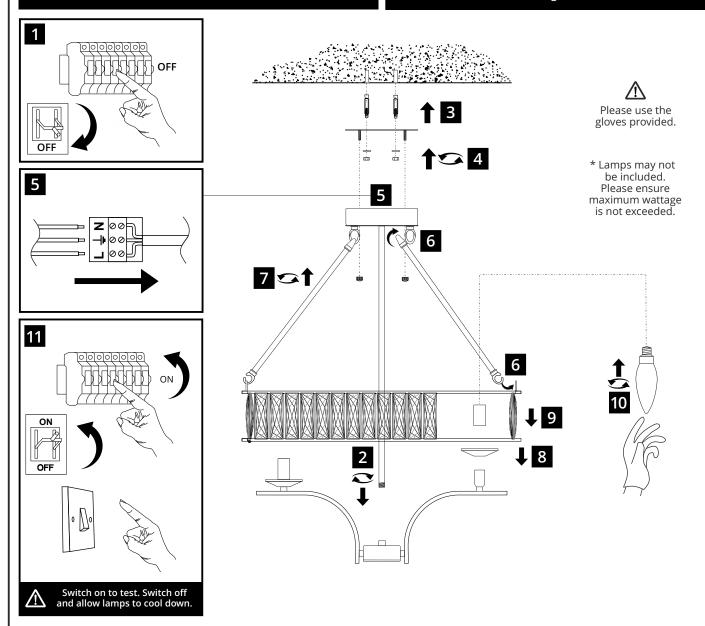
Voltage: 220-240V~50/60Hz Lampholder: E14/SES Lamps: 4 x LED 20W Max
