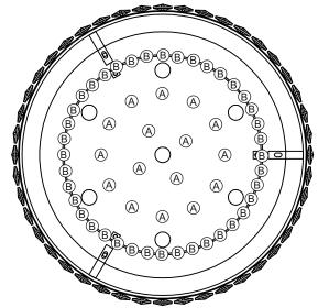
Voltage: 220-240V 50/60Hz Lampholder: G9 Lamps: 7 x 33W Max
