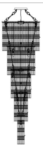
**Voltage:** 220-240V~50/60Hz Lampholder: E14/SES Lamps: 15 x 60W Max
