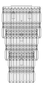
Voltage: 230V - 50/60Hz Lampholder: G9 Lamps: 4 x 33W Max
