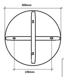
Inner bracket fixes to mounting surface. Fitting fixes to inner bracket.
