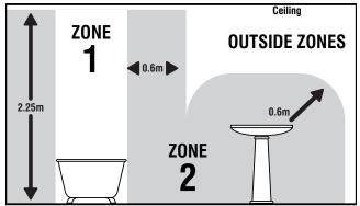
This product is suitable for use in Zone 2 and outside Zones of a bathroom. See diagram. If this unit is being fitted in a room containing a bath or shower, a 30mA RCD must be used, in accordance with IEE regulations.
